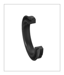
The profile E4 piston seal is a lip seal specially developed for use in pneumatics. The dimensions of the profile E4 standard series correspond to the cylinder diameters according to ISO 3320, CETOP RP 52 P, RP 43 P and RP 53 P. Profile E4 is fully interchangeable with the profile C2 standard series formerly used in pneumatics.
