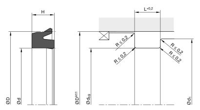
$d_1$  = minimum piston diameter on pressure side.
