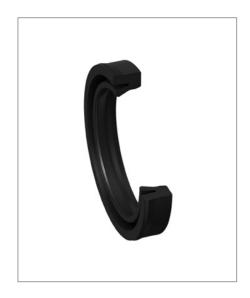
The profile E5 rod seal is a lip seal specially developed for use in pneumatics. The dimensions of the standard E5 profile series correspond to the rod diameters according to ISO 3320 and CETOP RP 51 P and are fully interchangeable with the C1 profile standard series formerly used in pneumatics.
