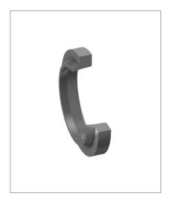
The function of the pneumatic wiper ring A2 is to prevent dust, dirt, grains of sand and metal shavings from entering the dynamic rod guide. This is achieved by a special design which largely prevents the development of dents, protecting the guiding parts, and extending the working life of the seals.
