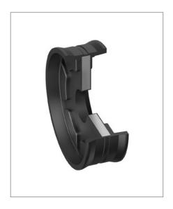
The double-acting profile DK is a complete pneumatic piston with a double cup seal and a vulcanized metal disc support. It performs two functions: **Sealing and guiding.**
