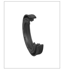
The Ultrathan® piston seal profile MK is a sealing element with integrated guiding and cushioning buffers. This seal-guide element can be used both on pistons with or without a permanent magnet. When used in magnetic pistons, the seal-guide element encapsulates the permanent magnet.
