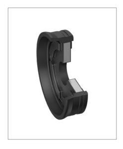
The single-acting profile EK is a complete pneumatic piston with a cup seal and a vulcanized metal disc support. It performs two functions:
