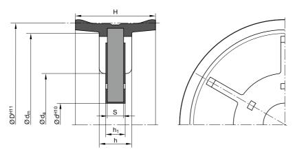
$\emptyset$  d<sub>m</sub> = max.  $\emptyset$  of joining metal parts
