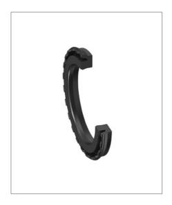
The profile Z8 cylinder seal is a single-acting lip seal for pistons in pneumatic cylinders and valves. It requires small housing dimensions. The standard series of profile Z8 conforms to the cylinder diameters of ISO 3320 and CETOP RP 52 P, RP 43 P and RP 53 P.
