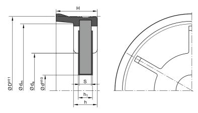
$\emptyset$  d<sub>m</sub> = max.  $\emptyset$  of joining metal parts
