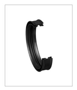
The profile Z5 pneumatic piston seal is a double U-ring with an integral guiding surface for double-acting pistons.
