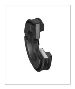
The double-acting profile DP is a complete pneumatic piston with a double cup seal and a vulcanized metal disc support. It performs three functions: **Sealing, guiding and cushioning.**
