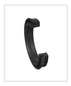
The profile E4 piston seal is a lip seal specially developed for use in pneumatics. The dimensions of the profile E4 standard series correspond to the cylinder diameters according to ISO 3320, CETOP RP 52 P, RP 43 P and RP 53 P. Profile E4 is fully interchangeable with the profile C2 standard series formerly used in pneumatics.
