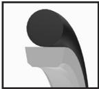
FROM double-acting rod sealing set. Particularly suitable for sealing rods in control cylinders, servo-assisted equipment and in quick-acting cylinders.
