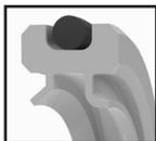
Flexilip rotary lip seal features an ID lip that seals dynamically on a shaft and an elastomeric o-ring on the OD to seal statically in a bore.
