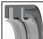
Flexicase rotary lip seal features an ID lip that seals dynamically on a shaft, and metal casing on the OD to seal statically press-fit into a bore.
