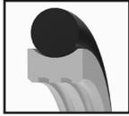
FTOR is suitable for applications where the pressure alternates from one side of the seal to another, such as pivots for rotating track rings, swivel joints, hose reels and in machine tool hydraulics.
