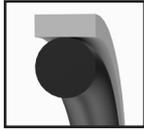
FPOA double-acting piston sealing set. Particularly suitable for double-acting pneumatic pistons. Assembly on one part piston is possible.
