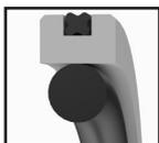
FPCQ double-acting sealing set is suitable for sealing between two media such as fluids/gases. Energised with an o-ring and incorporates an X-ring inset into the dynamic sealing face.
