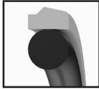
FPOD single-acting piston sealing set. Asymmetrical cross section is designed for best drag oil performance during stroke in both directions.
