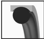
FPCR double-acting piston sealing set. Appropriate for dynamic applications as an alternative to an o-ring in situations where sealing performance and friction have to be optimised.
