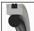
FPCQ with BU rings is used for higher pressure applications to prevent extrusion and can act as scraper function with more aggressive application media.
