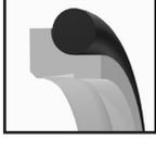
FWAD consists of a PTFE wiper ring and an elastomer o-ring as a pre-loading element. It combines two functions: wiping against pollution from outside and a sealing function which reduces the residual oil film.
