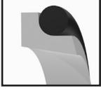
FWAT consists of PTFE wiper ring and elastomer o-ring as a pre-loading element. This profile is suitable for a wide range of applications, especially for aggressive media and/or high temperatures.
