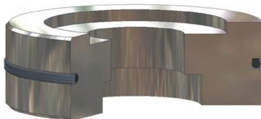
OQ installed in Rotary Gland
