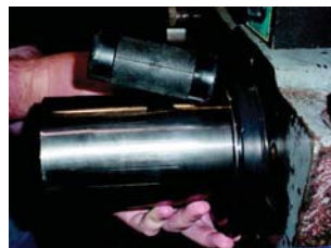
Installing the Seal
