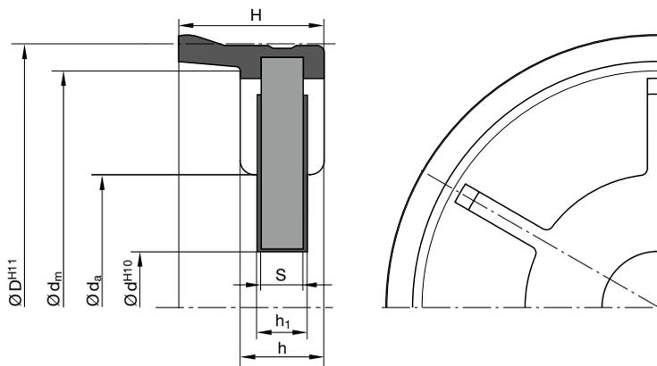
$\varnothing d_m = \text{max. } \varnothing \text{ of joining metal parts}$
