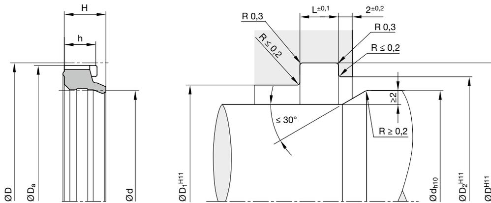
For surface finish, lead in chamfer and other installation dimensions see „General installation guidelines“.
