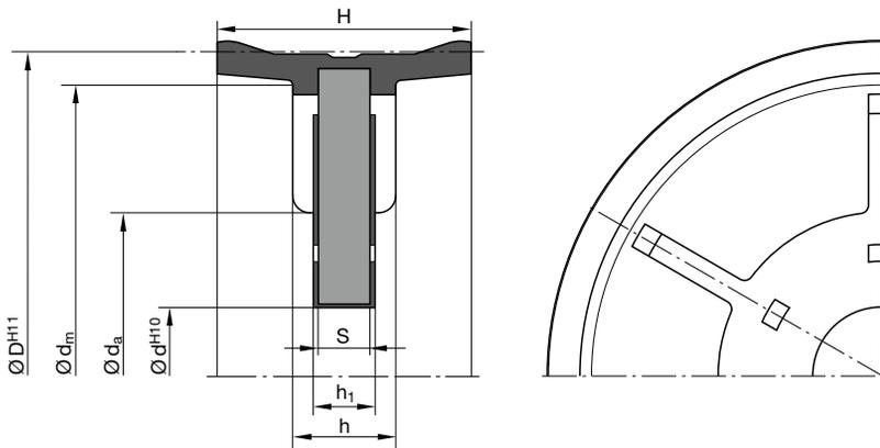
$\varnothing d_m$  = max.  $\varnothing$  of joining metal parts
