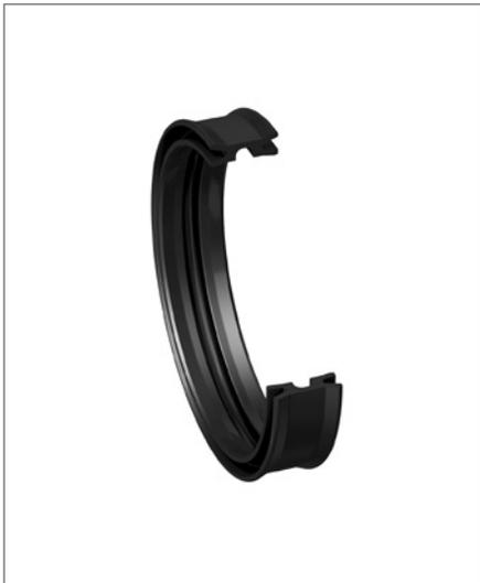
The profile Z5 pneumatic piston seal is a double U-ring with an integral guiding surface for double-acting pistons.
