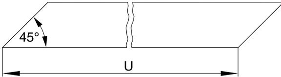
The length „U“ of the tape is to be calculated from the mean circumferential length less the clearance at the joint „k“. The k-values stated in the table are based on a temperature rise of 120 °C.
