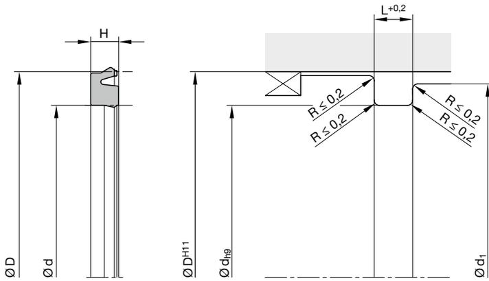
$d_1$  = minimum piston diameter on pressure side.
