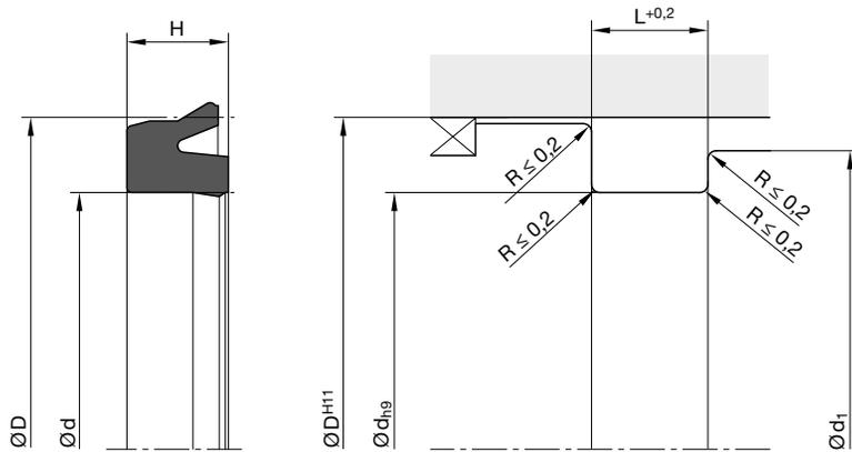
$d_1$  = minimum piston diameter on pressure side.
