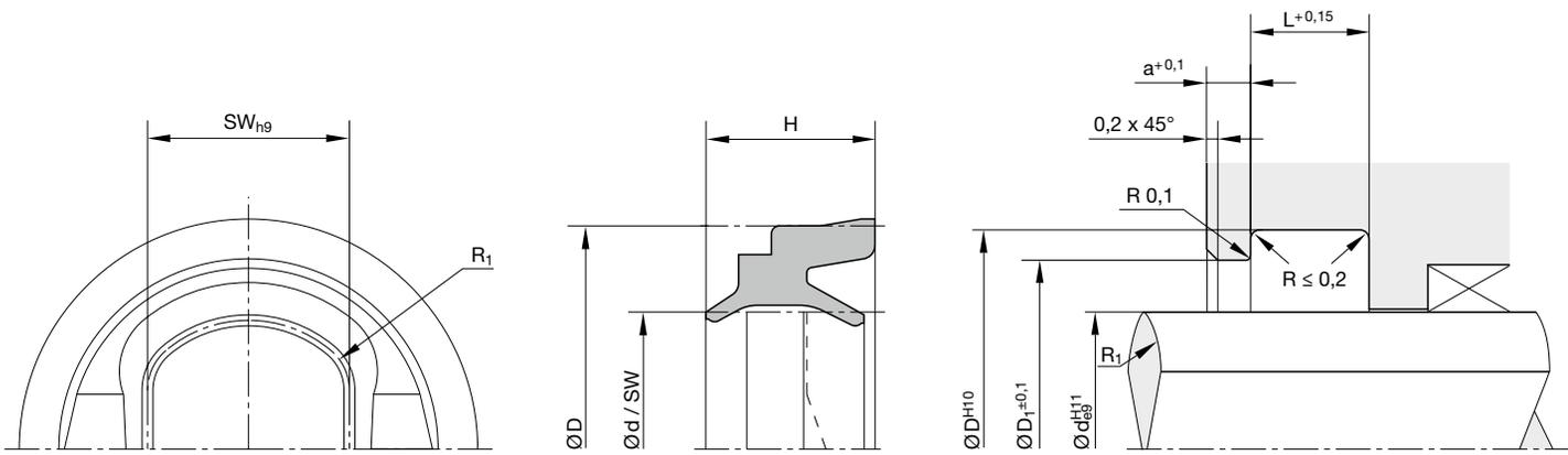
For surface finish, lead in chamfer and other installation dimensions see „General installation guidelines“.
