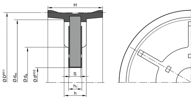
$\varnothing d_m$  = max.  $\varnothing$  of joining metal parts
