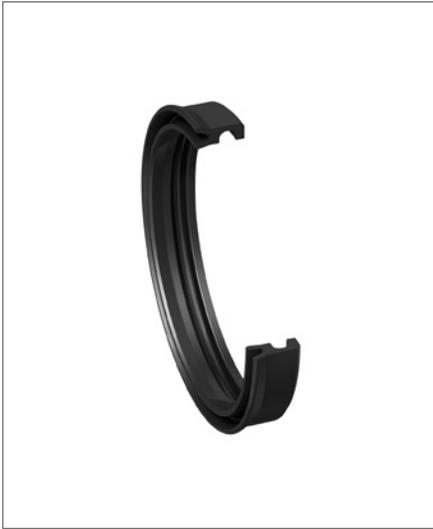
The profile Z7 pneumatic piston seal is a U-ring with an integral guiding surface for single-acting pistons.
