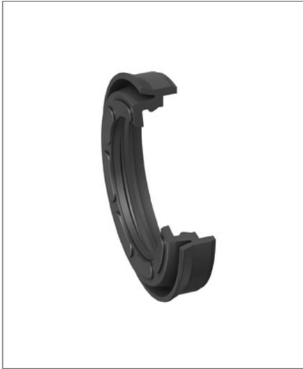
The Ultrathan® piston seal profile MK is a sealing element with integrated guiding and cushioning buffers. This seal-guide element can be used both on pistons with or without a permanent magnet. When used in magnetic pistons, the seal-guide element encapsulates the permanent magnet.
