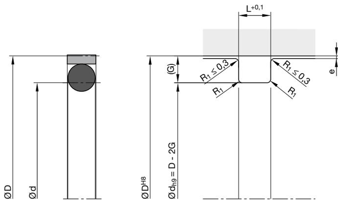
For surface finish, lead in chamfer and other installation dimensions see „General installation guidelines“.
