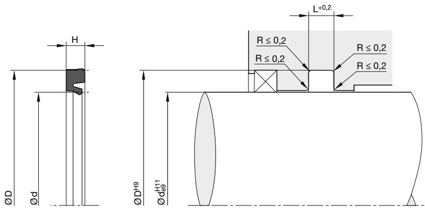
For surface finish, lead in chamfer and other installation dimensions see „General installation guidelines“.
