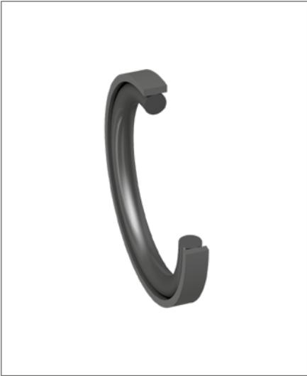
The double-acting piston sealing set profile OA consists of a PTFE piston sealing ring and an elastomer O-ring as a preloading element.
